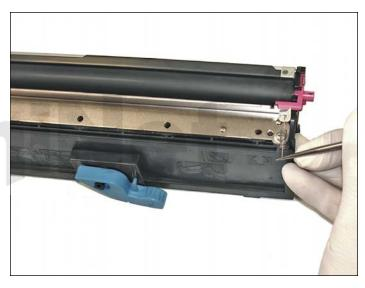
2. Using a hook tool, remove the two springs from the doctor blade. There is one at each end.
