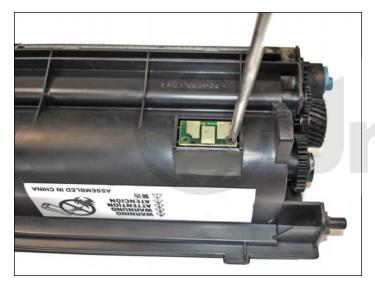
**REPLACING THE CHIP**
