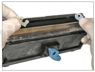
4. Remove the developer roller, lifting from the gear side first.
