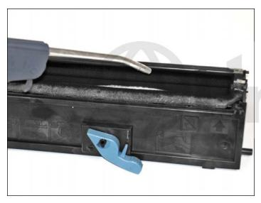
7. Using compressed air, thoroughly clean any residual toner from the hopper section. Make sure the sealing foam is properly installed to prevent toner leakage.
