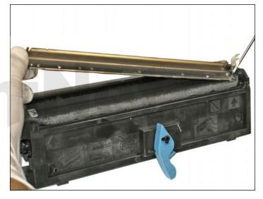
6. Remove the doctor blade, lifting from the gear side first.
